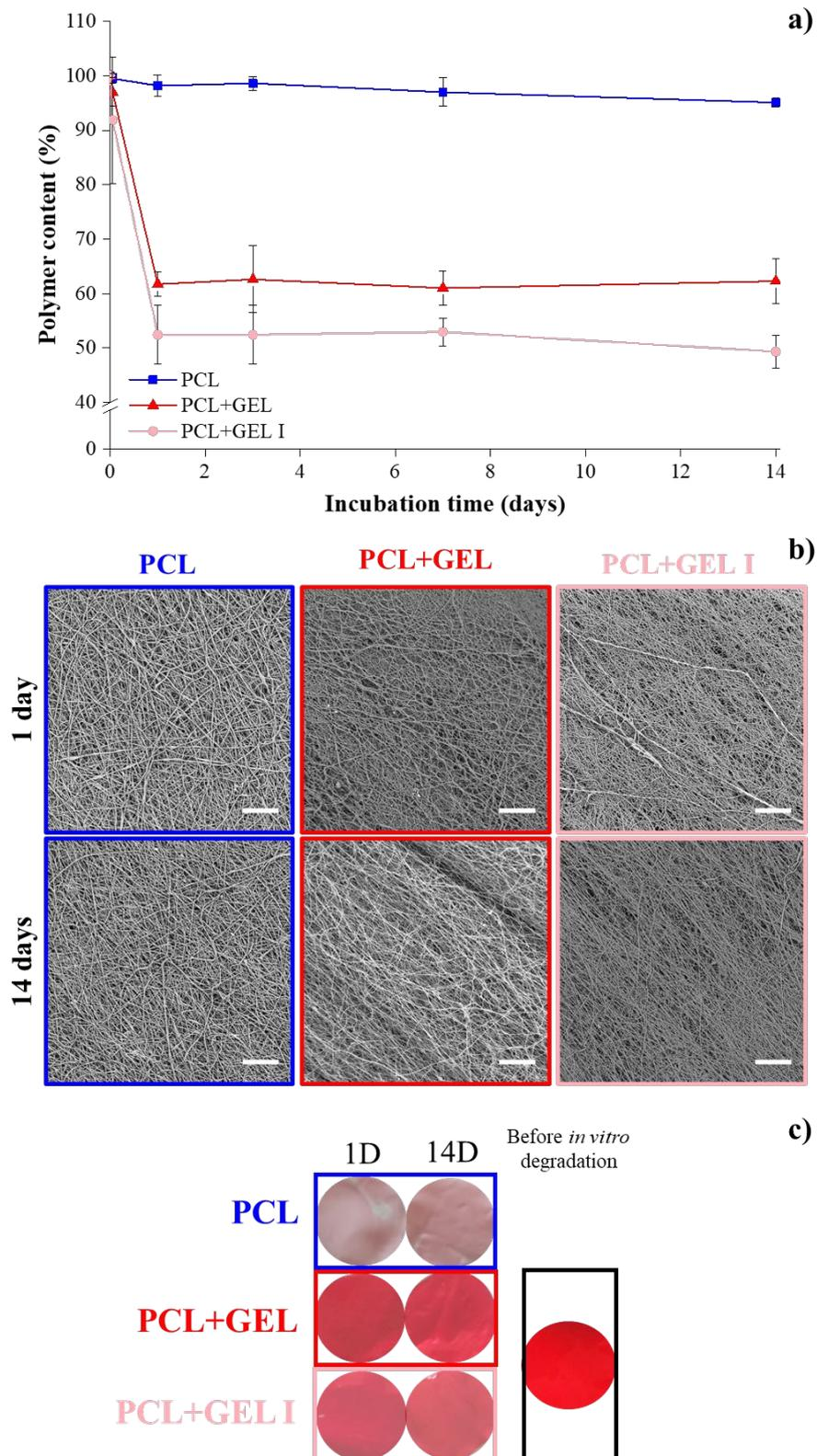
**Figure S2.** Polymer mass loss after biodegradation normalized to the polymer mass of PCL, PCL+GEL and PCL+GEL I (immersed only in PBS) (a), and the respective SEM images of the treated samples (b); Picrosirius red staining of PCL, PCL+GEL and PCL+GEL I scaffolds (c). Scale bar: 30  $\mu$ m.
