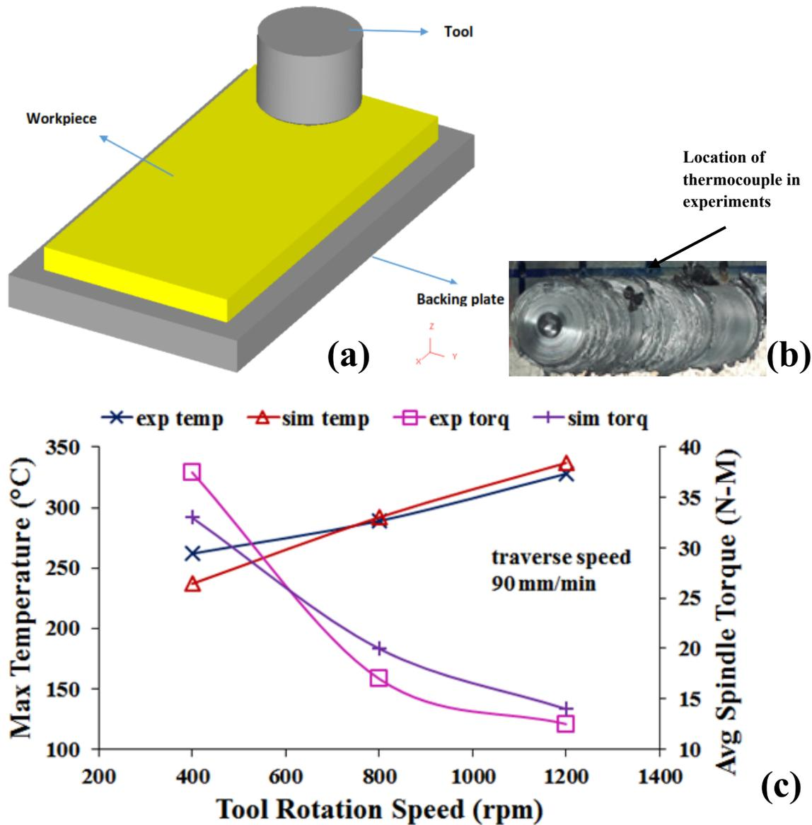
Figure 2. (a) FE model in DEFORM 3D (b) Photograph from experiments showing thermocouple location (c) Estimated and experimental values with trends for maximum temperature and average spindle torque for validation
