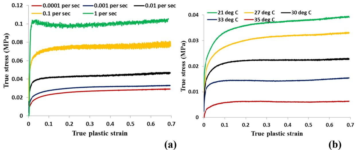
Figure 1. (a) True stress-true plastic strain curves obtained on plasticine deformed in compression at  $27^\circ\text{C}$  and at different strain rates. (b) True stress-true plastic strain curves obtained on plasticine deformed in compression at  $0.001\text{s}^{-1}$  and at different temperatures
