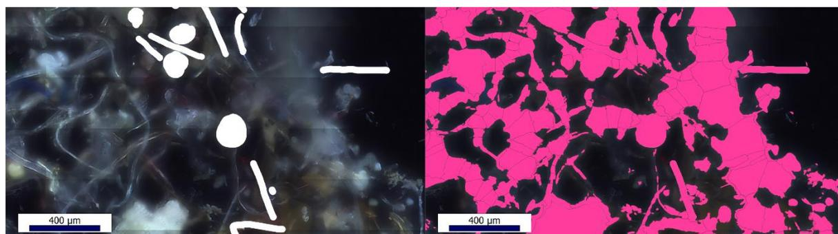
Figure S6: Detail of particle recognition of Filter 1. The white lines and blobs are drawn by hand to guide the watershed algorithm.
