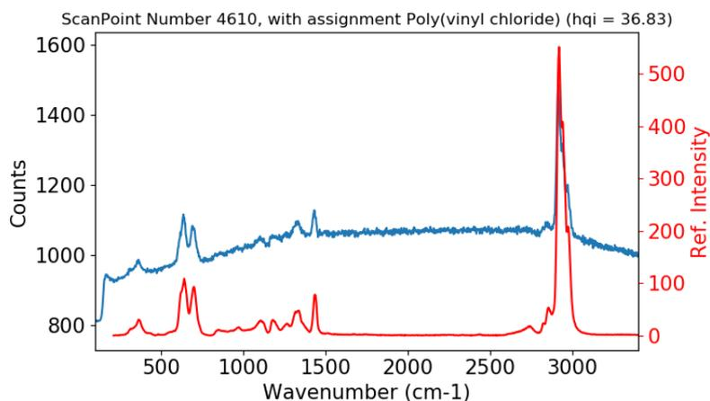
Figure S8. A spectrum of Poly(vinyl chloride) in the environmental sample (blue) together with the reference spectrum from the database (red).
