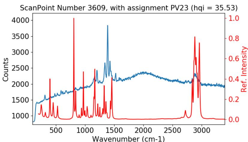
Figure S12. A spectrum of C. I. Pigment Violet 23 in a matrix of polypropylene in the environmental sample (blue) together with the polymer reference spectrum from the database (red).
