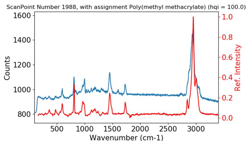
Figure S9. A spectrum of Poly(methyl methacrylate) in the environmental sample (blue) together with the reference spectrum from the database (red).
