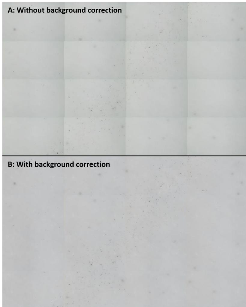
Figure S2. Effect of background correction during optical scan. Each tile represents an area of approx.  $500 \times 320 \mu\text{m}$ . Image A clearly shows the distinct shading artifacts from the inhomogeneous illumination of the sample. The artifacts were removed in Image B, making the subsequent particle recognition much more effective.
