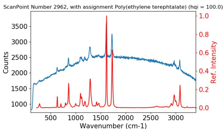
Figure S10. A spectrum of Poly(ethylene terephthalate) in the environmental sample (blue) together with the reference spectrum from the database (red).
