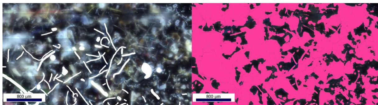
Figure S7: Detail of particle recognition of Filter 2. The white lines and blobs are drawn by hand to guide the watershed algorithm.
