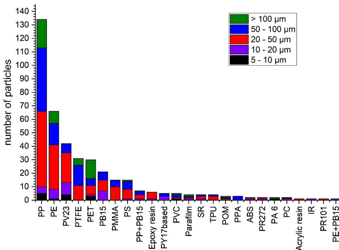
Figure S15. Overview over found MP particle distribution. PP = polypropylene, PE = polyethylene, PTFE = poly (tetrafluorethylene), PET = poly (ethylene terephthalate), PS = polystyrene, PVC = poly (vinyl chloride), SR = silicone rubber, TPU = Thermoplastic urethane, POM = polyoxymethylene, PPA = polyphthalamide, ABS = acrylonitrile butadiene styrene, PA = polyamide, PC = polycarbonate, IR = isoprene rubber, PB = pigment blue, PV = pigment violet, PY = pigment yellow, PR = pigment red.
