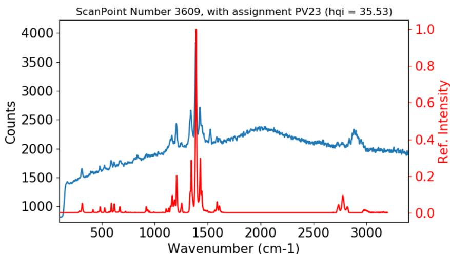
Figure S11. A spectrum of C. I. Pigment Violet 23 in a matrix of polypropylene in the environmental sample (blue) together with the pigment reference spectrum from the database (red).
