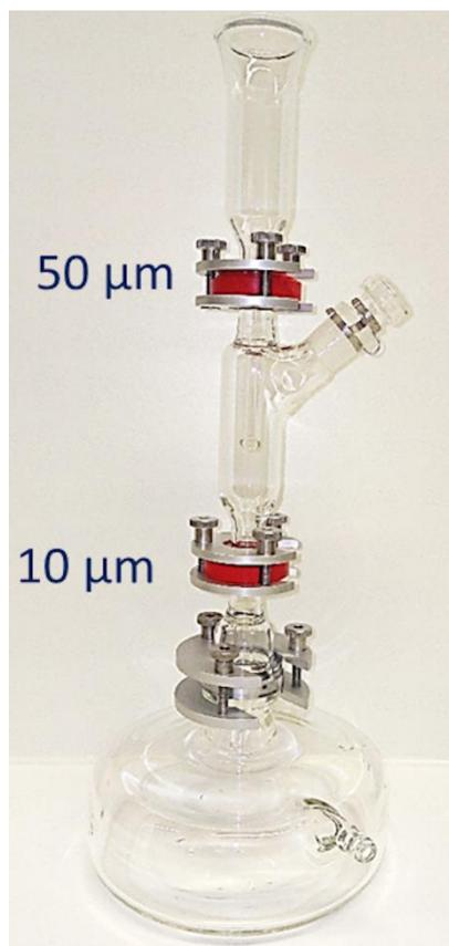
Figure S16. Glass filtration apparatus for realizing a fractionated filtration.
