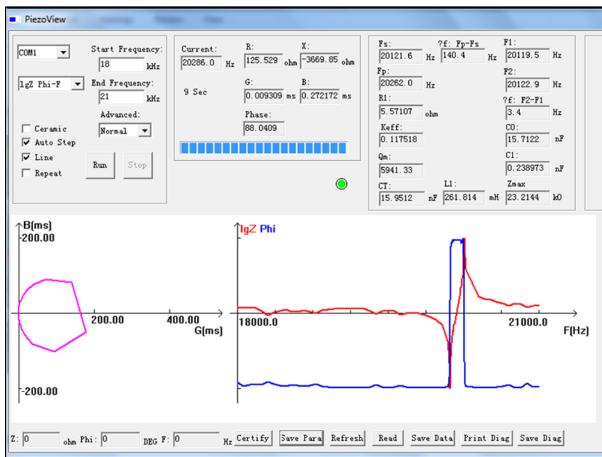
Figure S1: Measurement of vibrational frequency using a PiezoView software, of the designed tool assembly
