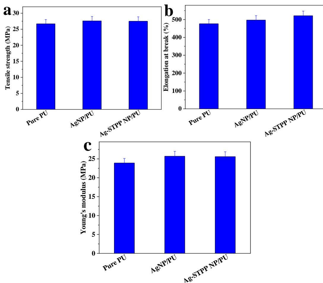
**Figure S3.** Mechanical properties: (a) tensile strength, (b) the elongation at break, (c) Young's modulus.
