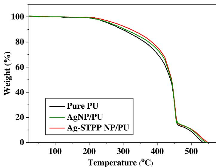
**Figure S2.** TGA image of the pure PU film, AgNP/PU and Ag-STPP NP/PU.
