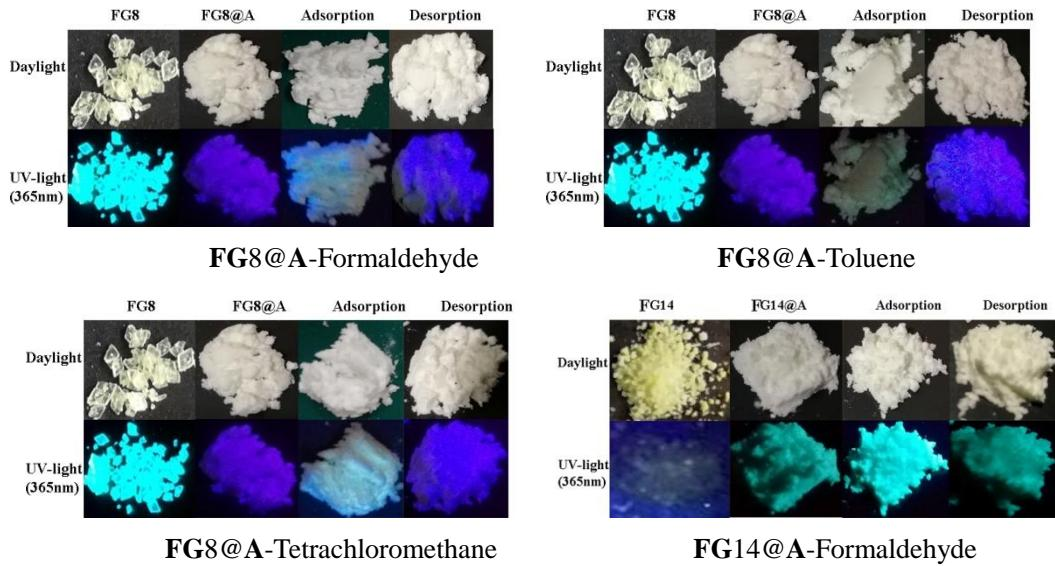
**Fig. S26.** A comparison of fluorescence changes of the selected FG8 or 14@A adsorbing and desorbing the selected volatile compounds.
