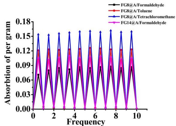
**Fig. S24.** Lifetime experiments of adsorption capacities of two selected solid **FG8@A** and **FG14@A** for selected volatile compounds.
