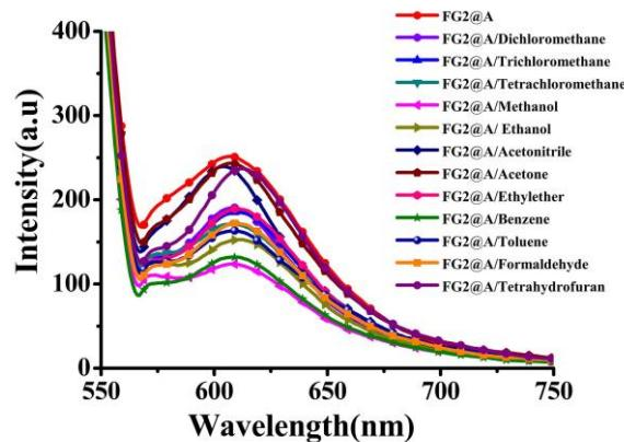
**Fig. S6.** General survey of fluorescence spectra of FG2@A loaded with the 12 respective VOCs.
