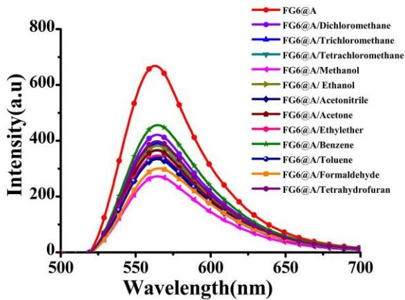
**Fig. S10.** General survey of fluorescence spectra of FG6@A loaded with the 12 respective VOCs.
