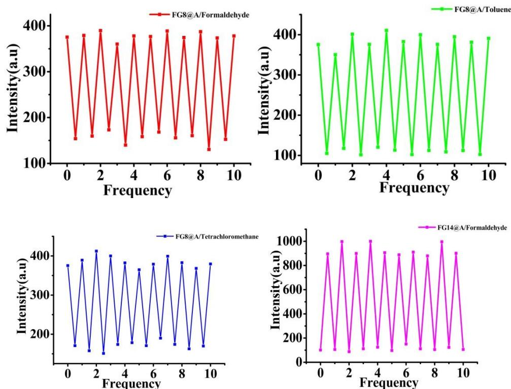
**Fig. S25.** Lifetime experiments of fluorescence strength of solid **FG8@A** and **FG14@A** for the selected volatile compounds.
