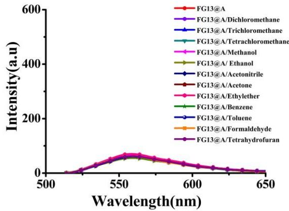
**Fig.S17.** General survey of fluorescence spectra of FG13@A loaded with the 12 respective VOCs.
