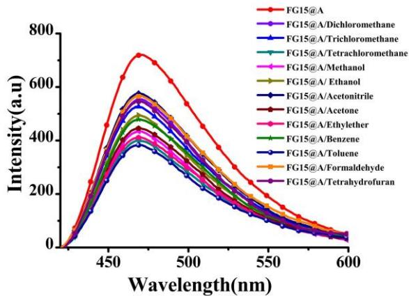
**Fig. S19.** General survey of fluorescence spectra of FG15@A loaded with the 12 respective VOCs.
