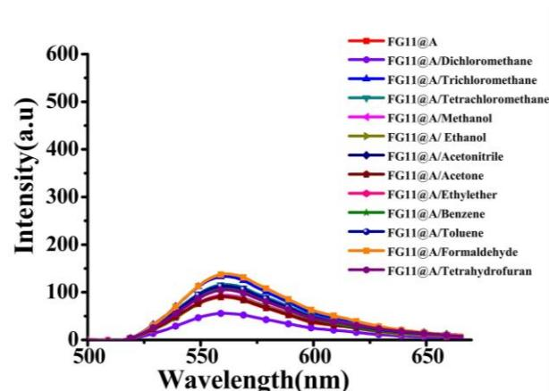
**Fig. S15.** General survey of fluorescence spectra of FG11@A loaded with the 12 respective VOCs.
