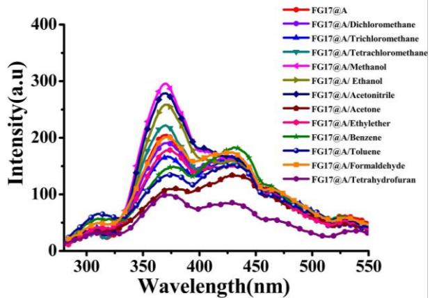
**Fig. S21.** General survey of fluorescence spectra of FG17@A loaded with the 12 respective VOCs.
