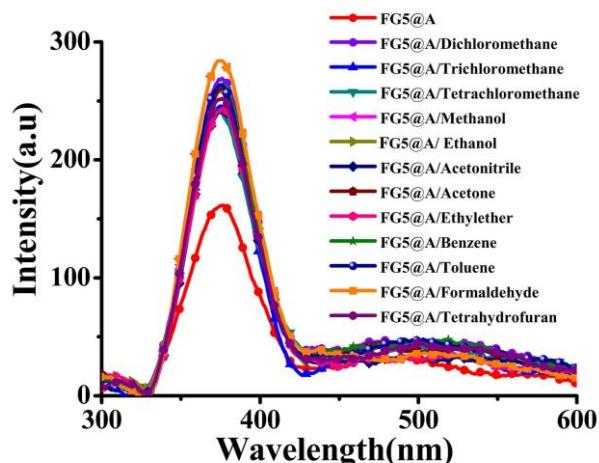
**Fig. S9.** General survey of fluorescence spectra of FG5@A loaded with the 12 respective VOCs.
