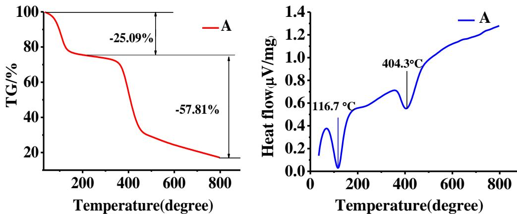
**Fig. S3.** TG (left) and DTA (right) curves of A in  $\text{N}_2$ .
