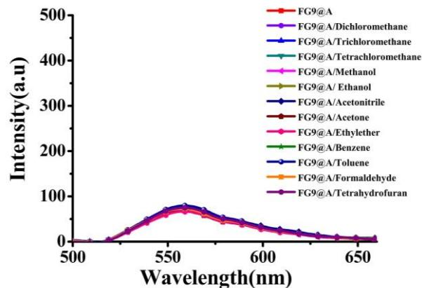
**Fig. S13.** General survey of fluorescence spectra of FG9@A loaded with the 12 respective VOCs.
