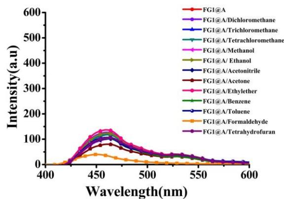
**Fig. S5.** General survey of fluorescence spectra of FG1@A loaded with the 12 respective VOCs.
