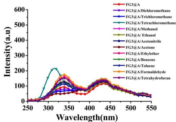
**Fig. S7.** General survey of fluorescence spectra of FG3@A loaded with the 12 respective VOCs.
