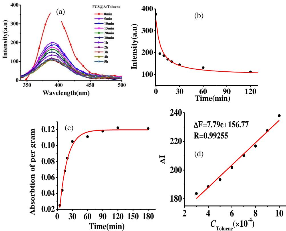
**Fig. S22.** (a) Titration fluorescence spectra of the loading of **FG8@A** with toluene; (b) change in fluorescence intensity of **FG8@A** with increasing adsorption time; (c) adsorption profile of the loading of toluene in **FG8@A**; (d) plot of  $\Delta I$  vs. the amount of toluene adsorbed by solid **FG8@A**.
