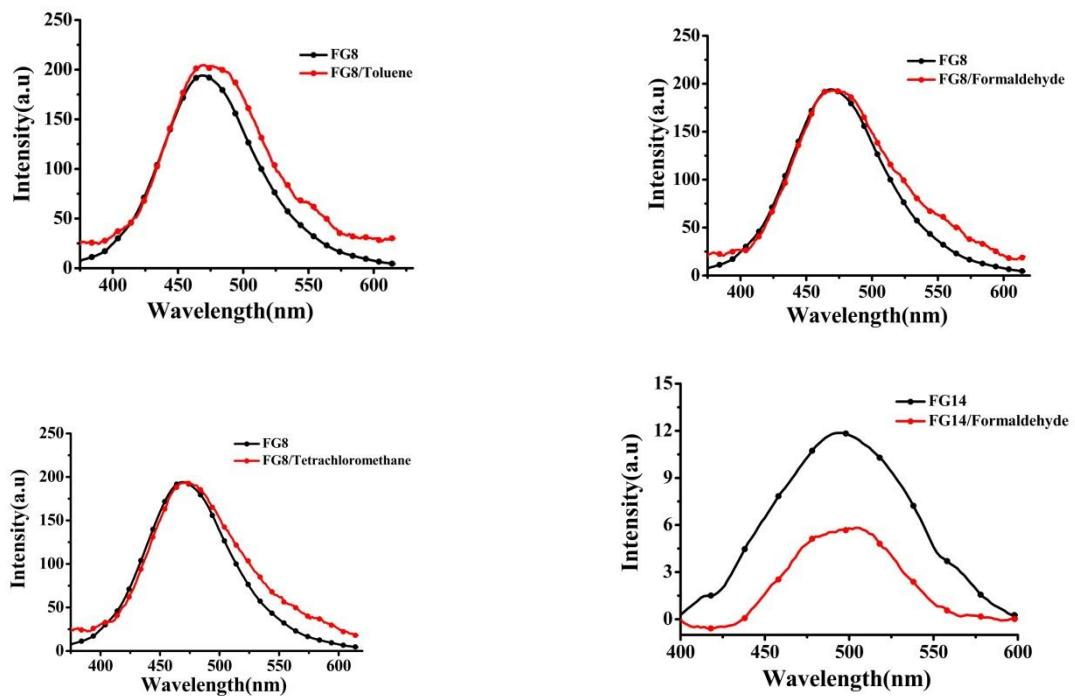
**Fig. S27.** Influence of the selected volatiles compounds absorbed by neat FG8 and FG14 on the fluorescence strength of the FG8 and FG14, respectively.
