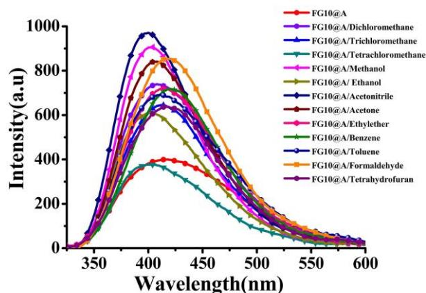
**Fig. S14.** General survey of fluorescence spectra of FG10@A loaded with the 12 respective VOCs.
