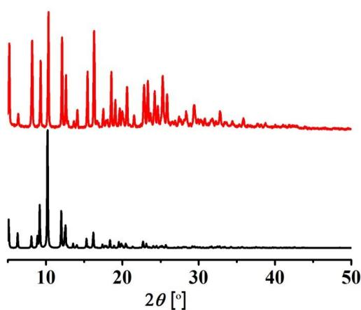
**Fig. S2** Powder X-ray diffraction analyses of A (top) and comparison with simulation (bottom)
