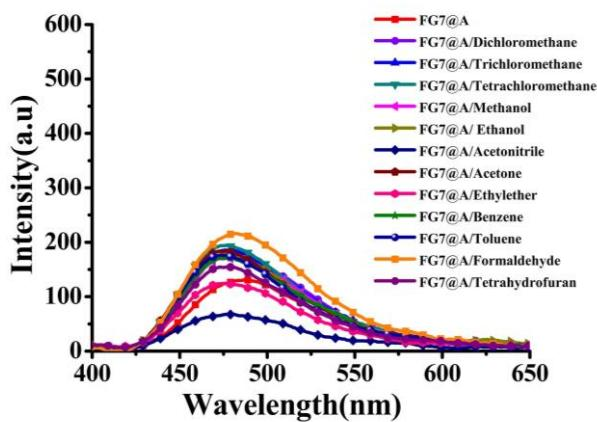
**Fig. S11.** General survey of fluorescence spectra of FG7@A loaded with the 12 respective VOCs.
