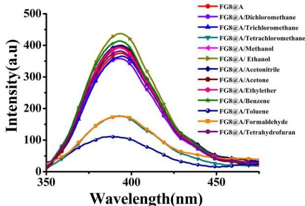
**Fig. S12.** General survey of fluorescence spectra of FG8@A loaded with the 12 respective VOCs.
