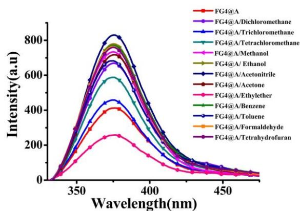
**Fig. S8.** General survey of fluorescence spectra of FG4@A loaded with the 12 respective VOCs.
