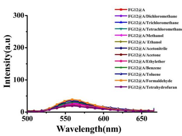
**Fig. S16.** General survey of fluorescence spectra of FG12@A loaded with the 12 respective VOCs.
