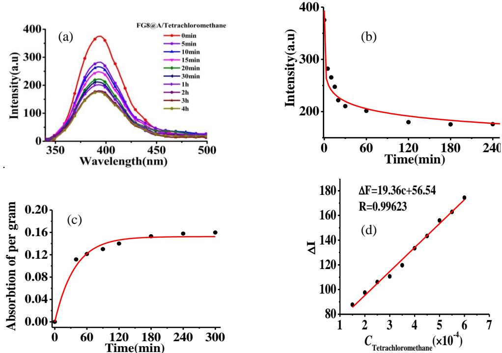
**Fig. S23.** (a) Titration fluorescence spectra of the loading of **FG8@A** with tetrachloromethane; (b) change in fluorescence intensity of **FG8@A** with increasing adsorption time; (c) adsorption profile of the loading of tetrachloromethane in **FG8@A**; (d) plot of  $\Delta I$  vs. the amount of tetrachloromethane adsorbed by solid **FG8@A**.
