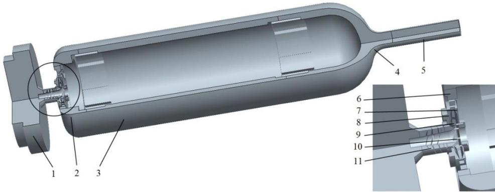
1.Foundation chamber 2.Middle section chamber 3.Outer cylinder chamber 4.Channel of casing cover 5.Outlet duct
