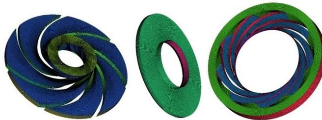
(a) impeller mesh (b) back chamber mesh (c) guide vane mesh
