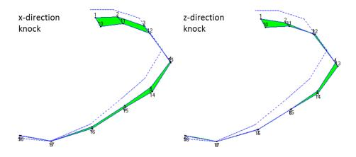
Figure S1: First bending mode of 1LO at 3.94Hz and 3.90Hz with free-free boundary condition knocked in X&Z-direction respectively
